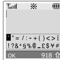
Use the navigation keys to scroll to the required symbol and then press the **OK** soft key to insert the highlighted symbol into your message.
