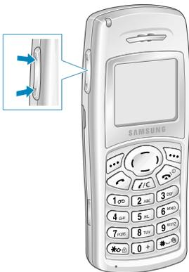
In idle mode, you can adjust the key volume using the same keys.
