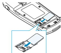
**Note:** When you need to remove the SIM card, slide it, as shown below, and take it out of the holder.
