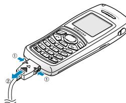
**Note:** Do not remove the battery from the phone while it is charging without first unplugging the adapter. If you do so, the phone may be damaged.
